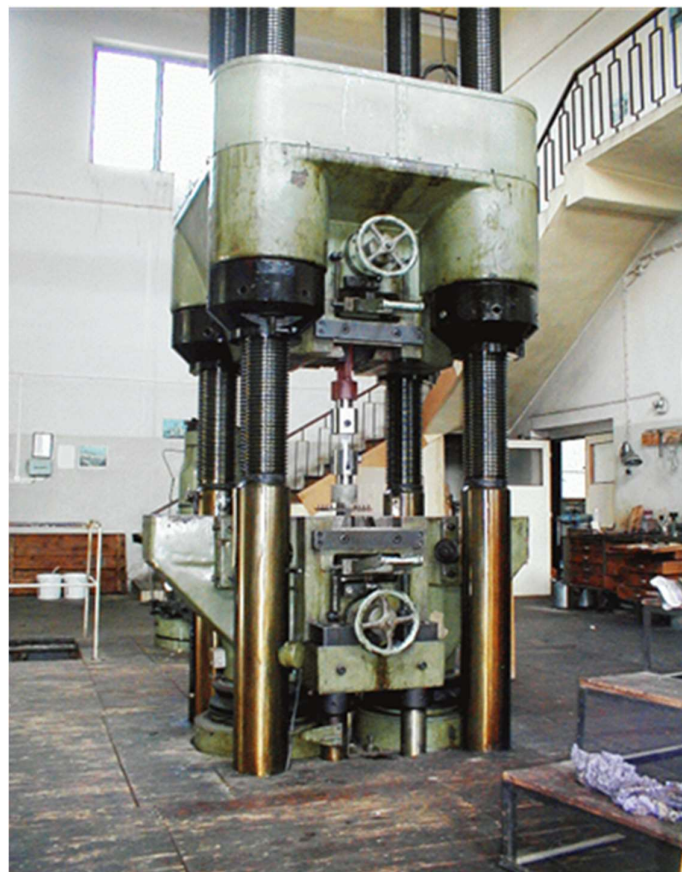
Fig. 7. Pulsator with loading capacity of 6000 kN adopted
