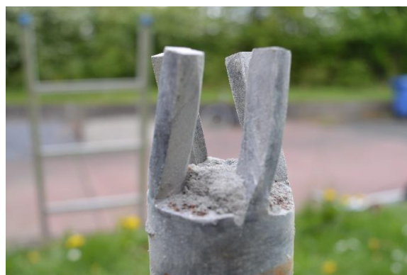
Figure 14. Excessive bending of strips
