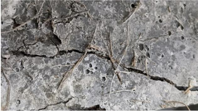
Figure 14. Failure pattern of fiber reinforced beam specimen
