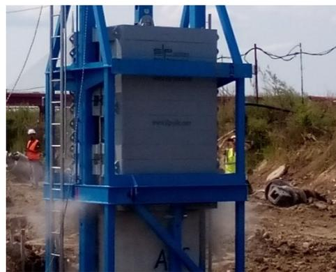
Figure 6. Testing by 42t falling weight from the elevation of 0.3 to 1.5m
