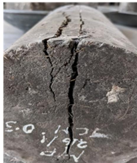
Figure 10. Failure pattern of fiber reinforced cylinder specimen
