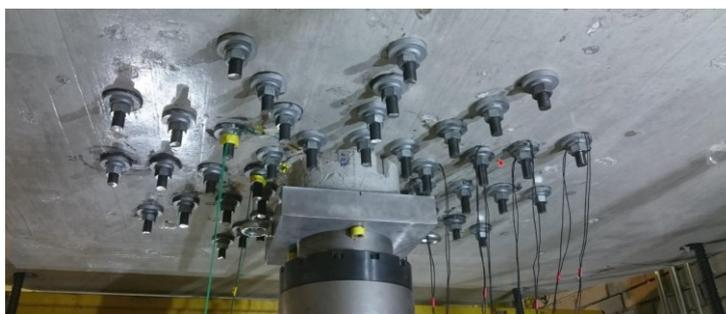
Figure 3. Large scale punching shear tests [1]
