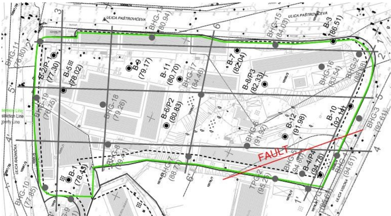
Figure 37. The direction of the fault in zone 2 and the transition from limestone breccias to clays
