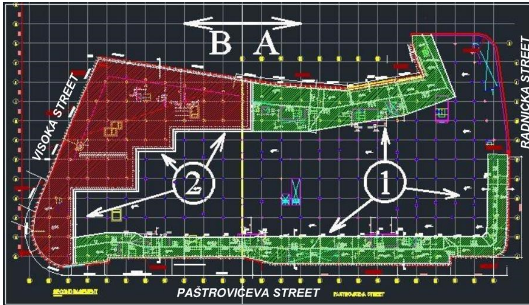
Figure 4. Construction Plan - division of the building into part A and B and application of two types of top-down methods 1 and 2
