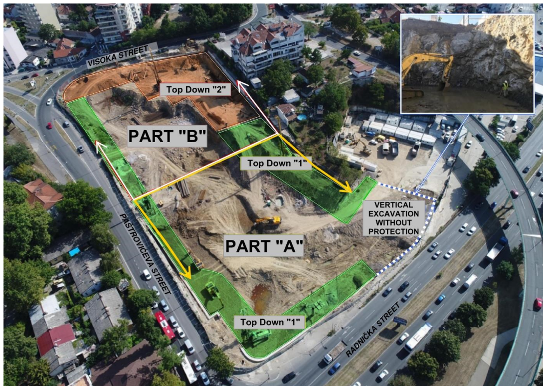
Figure 5. Construction Plan - division of the building into parts A and B and application of two types of top-down methods 1 and 2
