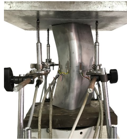
Figure 1. Typical stub column failure mode [1]
