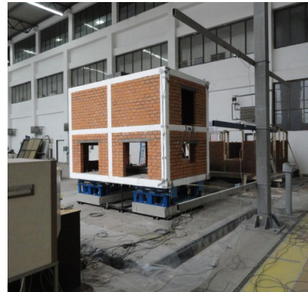
Figure 13. Testing of the HC-RMS-GOSEB system: (Model in DYN-LAB) IZIIS-Skopje
