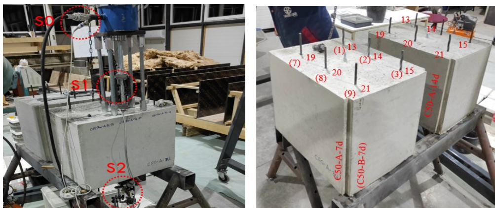
Figure 8. Test arrangement and position of the sensors (left) and concrete specimens with numbering (right)
