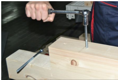
Slika 6. Priprema ojačanih uzoraka Figure 6. Preparation of reinforced specimens
