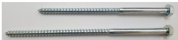
Slika 3. Zavrtnji za ojačanje Figure 3. Screws used as reinforcement
