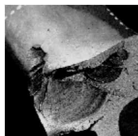
Slika 11. Lom šine usled razvoja head checking defekta Figure 11. Rail break caused by the head checking
